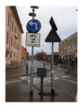
Working in partnership with Solagen, a UK supplier of safety warning signs, Q-Free integrated the HI-TRAC CMU with a solar-powered flashing sign on one of the main commuter corridors. Upon detection of a cyclist, a signal is sent to the sign, which flashes a warning to oncoming motorists until the cyclist is safely through the junction.
