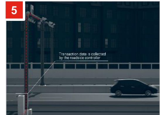
Processing of data from cameras, transceivers/ tags and vehicle detectors in Q-Free's roadside controller, submission of relevant data to central back-office system for billing and reporting
